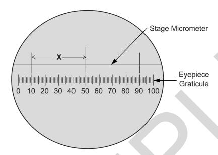
(i) The distance **X** on the stage micrometer is **0.1 mm**.
