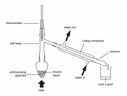
In both distillation and heating under reflux, antibumping granules are added to the reaction mixture. These act as nucleation sites for bubbles, ensuring that the liquid boils smoothly.
