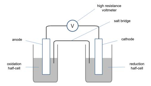
A diagram of a typical electrochemical cell is shown above. The direction of electron flow in the diagram is from the anode to the cathode.
