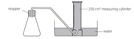
During this procedure, some gas produced will be lost as the stopper is replaced after adding reagents. Additionally, some of the carbon dioxide will dissolve in the water, so the volume of carbon dioxide collected will be less than expected. Both of these factors lead to the calculated percentage by mass of copper(II) carbonate being smaller than would otherwise be expected.
