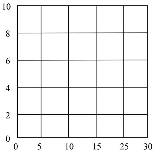
Not acceptable - non-linear scale on the x-axis
