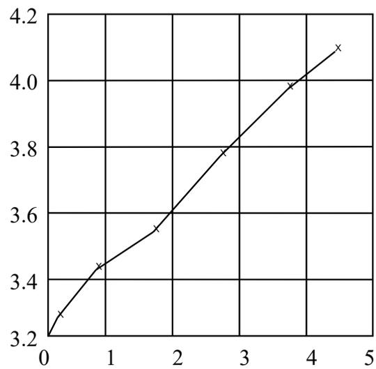
Not acceptable – joining point-to-point
