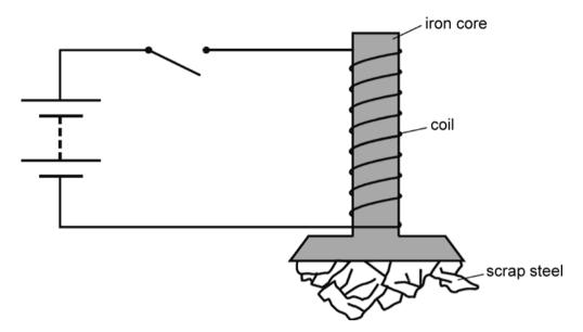
When the switch is closed, the scrap steel is attracted to the electromagnet.
