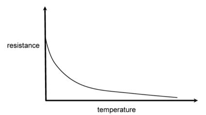
(a) What happens to the resistance of the thermistor as the temperature increases?
