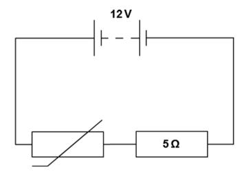
A current of 2 A flows through the 5  $\Omega$  resistor.
