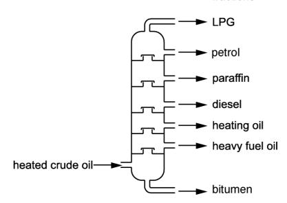
(a) Crude oil contains a mixture of hydrocarbons that boil at different temperatures.
